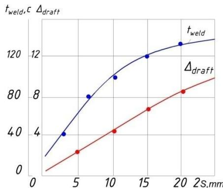
Fig. 4. Dependence of draft  $\Delta_{draft}$  and welding time on the thickness of the welded strips  $2s$
