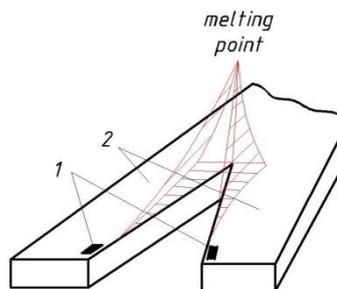
Fig. 1. Scheme of the process of high-frequency pressure welding with reflow:
