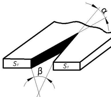
Fig. 2. Symmetric scheme of high-frequency welding of longitudinal pipes
