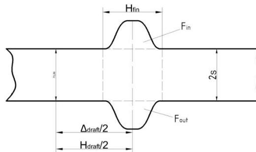
Fig. 3. Scheme for determining precipitation
