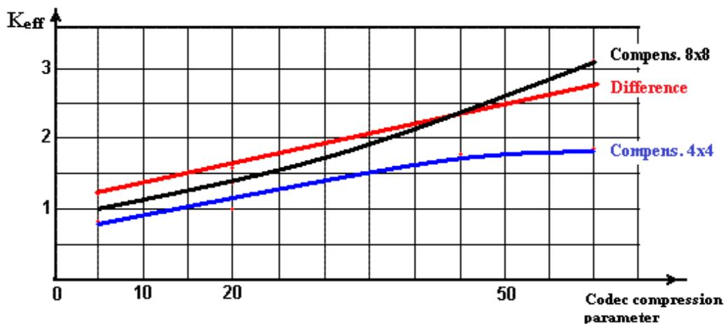
Fig. 7. Evaluation of the effectiveness of interframe processing options when compressing the Road video plot
