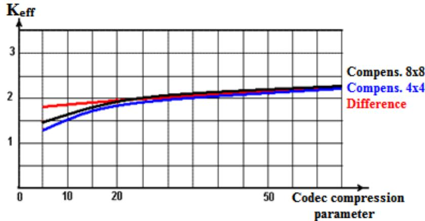
Fig. 10. Evaluation of the effectiveness of inter-frame processing options when compressing the Post video plot
