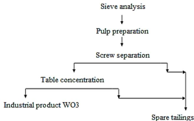
**Fig.№ 1. The technological scheme of enrichment of the tailings of the Ingichkin factory by the gravitational method in an open cycle.**
