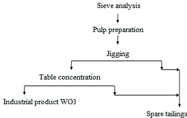
The following 3 experiments were also carried out in an open cycle according to the following flow chart:
