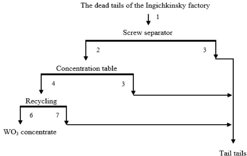
**Fig. 4 Technological scheme of enrichment of the tailings of the Ingichkin factory by the gravitational method.**
