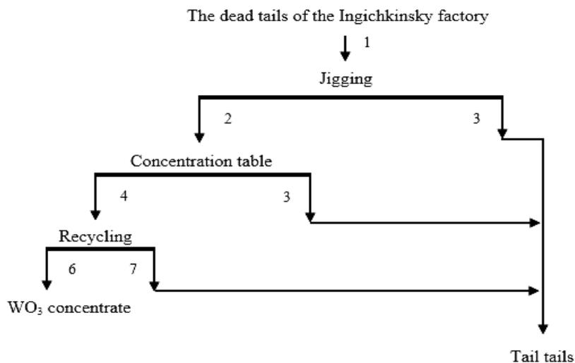
**Fig. 3 Recommended technological scheme of enrichment of the tailings of the Ingichkinsky factory by the gravitational method.**
