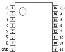
Figure 6: Pin Configuration of 74HC151
