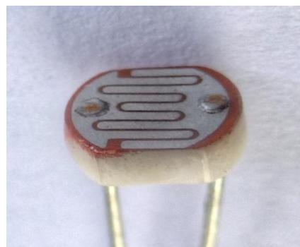
Figure 5: Optical Sensor (LDR)
