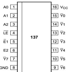
Figure 10: Pin Configuration of 74HC137
