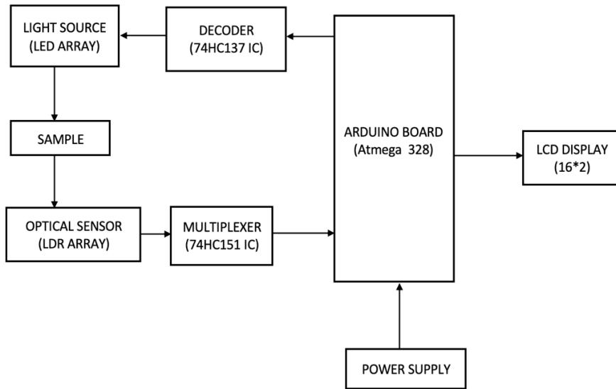
Figure 11: Block diagram
