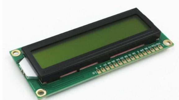
Figure 2: Liquid crystal display(16x2)
