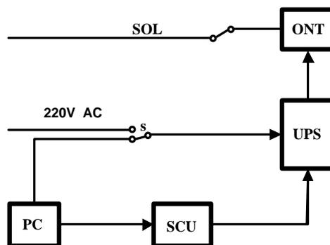
Fig 3. Autonomous power supply of ONT subscriber devices
