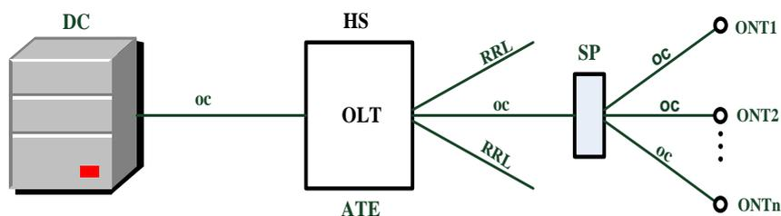
Fig 1. Model of a fragment of a rural (RTN) built on the basis of PON technology.
