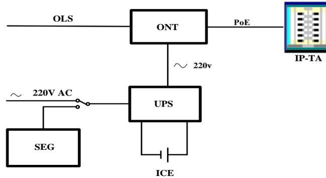
Fig 2. Organization of uninterrupted power supply at the subscriber level
