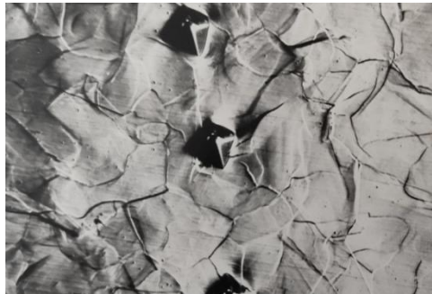
c) x500 Fig. 4. The deformation relief arising at a temperature of 870 0 C. (ЗГП - grain boundary slippage. BC - intragranular slip)
