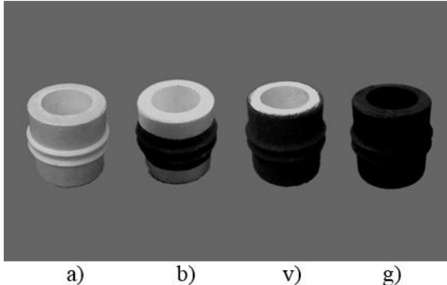
**Fig.1. Foam models of rollers of rolling mill No.KB-10.5287 with wear-resistant carbide coating: a-foam model; b-foam models with coating on the main wearing surfaces; v-foam models for the entire wear surface; g-cast steel parts of the harrow and roller teeth with carbide coating and subsequent thermal hardening.**
