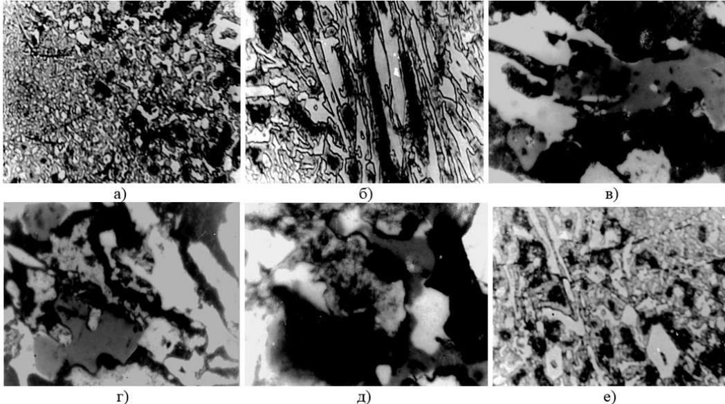
**Fig. 2.** Cross section with small carbide particles (a) and longitudinal section with brittle chipping (b) X300 and microstructure of sulfides (c); spalling of sulphide particles and the formation of a weakened zone at the phase boundaries (d) of X1700 and the microstructure of sulphide particles of phases (e) and iron carbide (e). X1700
