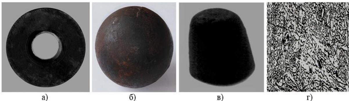
**Fig. 3.** Finished cast parts cast from high-chromium white cast iron: a-pump impeller; b-ball drum; b-clippers of the drum; g-microstructure of fine carbide white cast iron. X500
