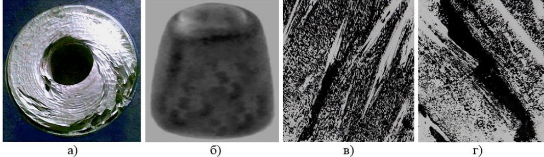
Fig. 1. Cast worn parts and macrostructures cast from high-chromium white cast iron: a-pump impeller; b-clippers of drum mills; c, g-cracked specimens.
