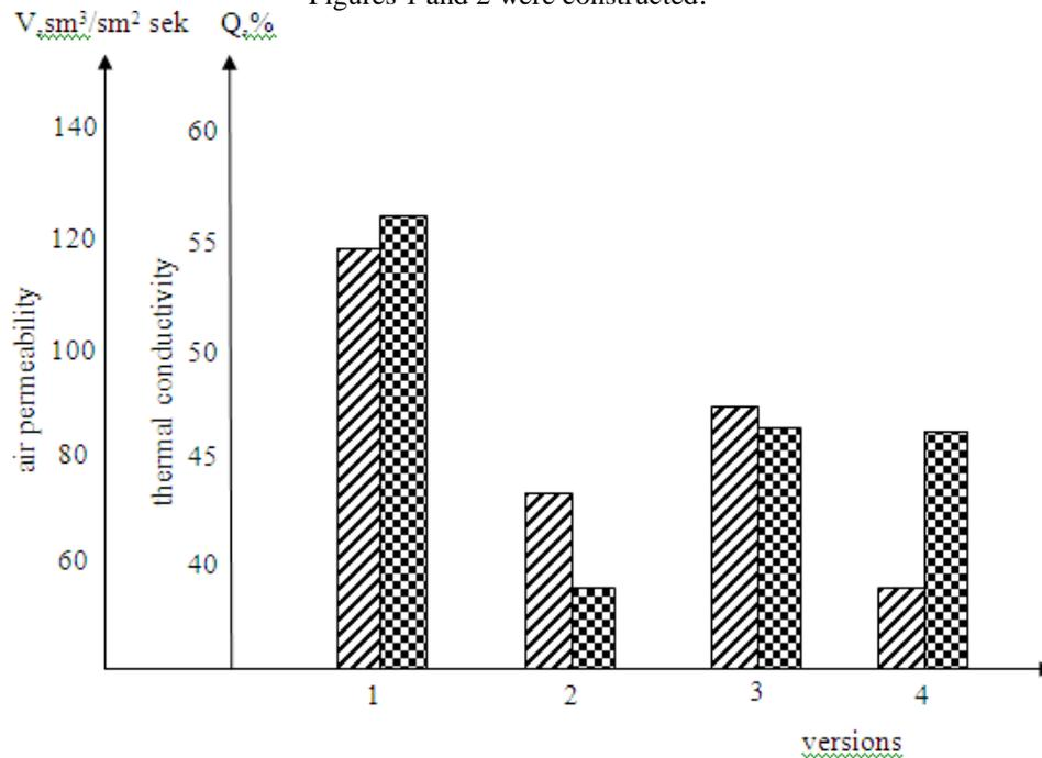
Figure 1. Air and heat of non-woven fabrics' change in conductivity.
