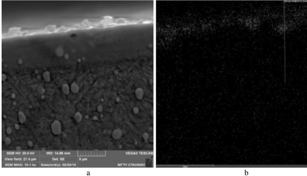
**Fig.4. Zirconium nitride modified subsurface layer of high-speed M2 steel. (a) SEM-image of the etched specimen, (b) map of the distribution of zirconium in the specimen.**
