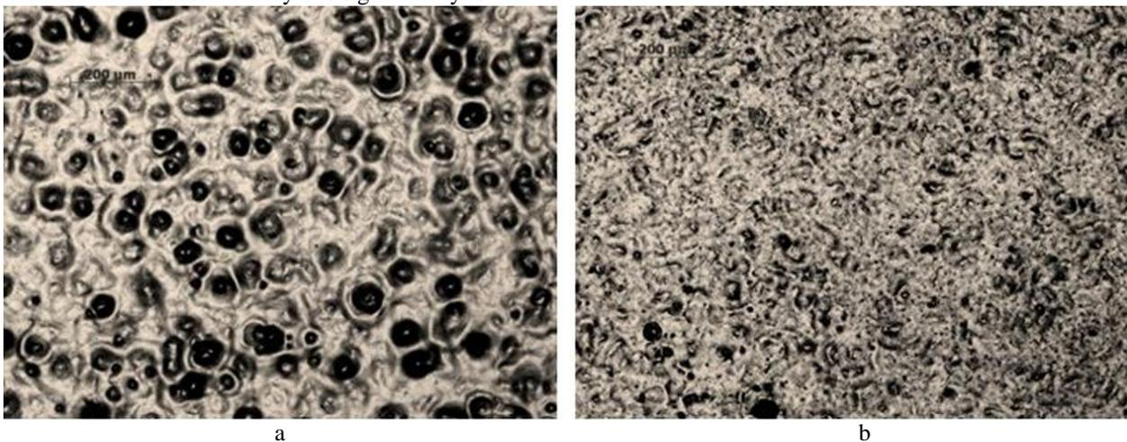
**Fig.2. (a) Structure of nitride high-speed M2 steel surface after exposure to LEHCEB, (b) The same, after electron-beam zirconium-alloying.**
