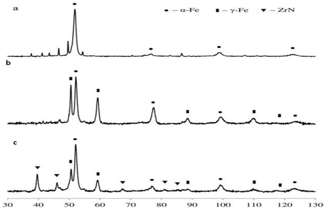
Fig.3. (a) Diffraction pattern (CoK $\alpha$ ) of nitride M2 steel specimen surface, (b) the same, after exposure to LEHCEB, (c) the same, after applying Zr coating on the surface before irradiation.
