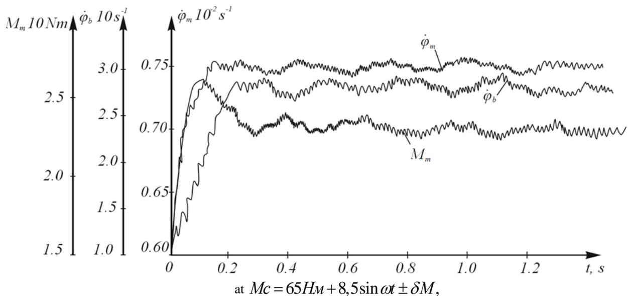
Fig. 3. The patterns of change in the angular velocity of the rotor of the engine, the screw shaft, as well as the torque on the motor shaft.
