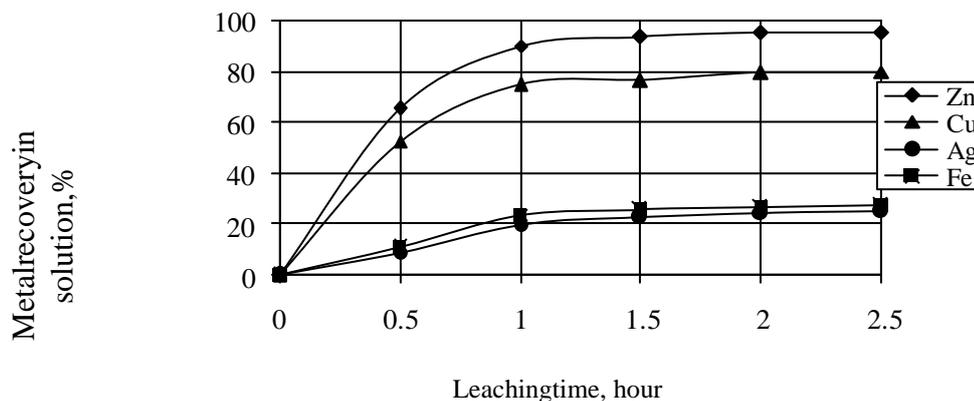
Fig. 2. Dependence of the degree of extraction of metals into the solution on the duration of leaching.
