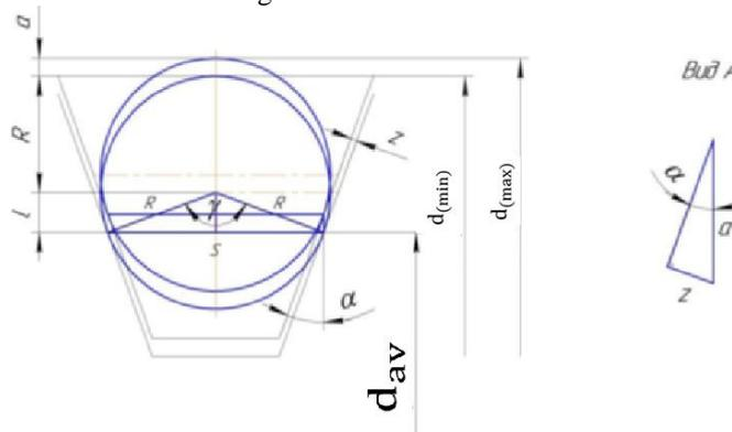
Fig.3 Determination of allowance.
