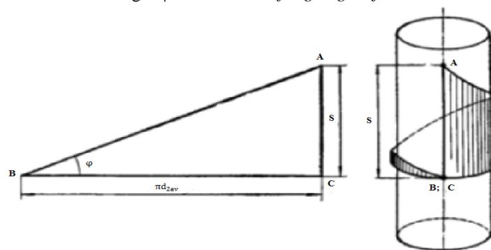
**Fig 1. Formation of a helical surface**
