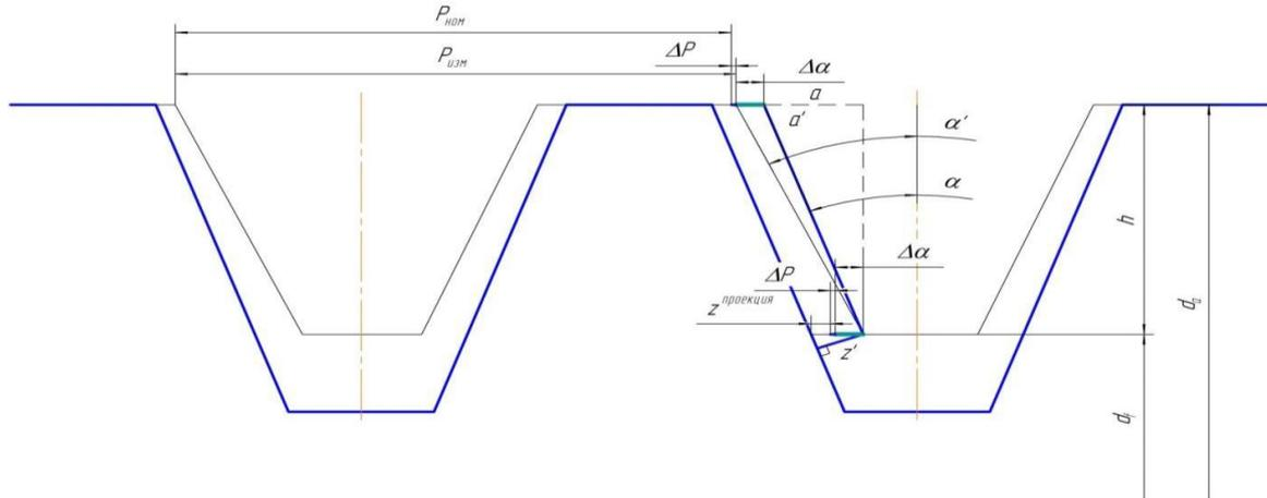
Fig. 4. Profile draft for building a dimensional chain.
