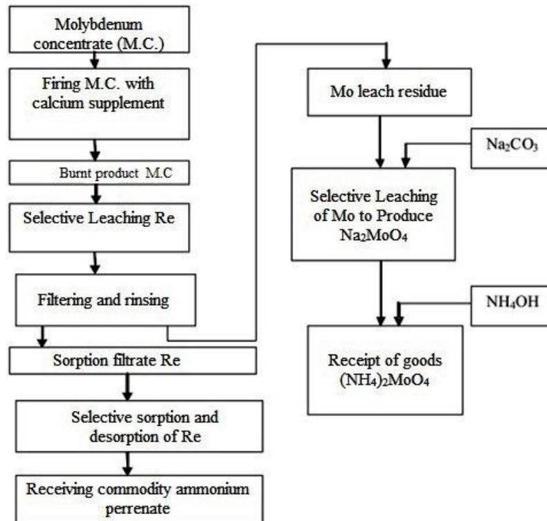
Fig. 1. Schematic diagram of the processing of non-standard molybdenite concentrates
