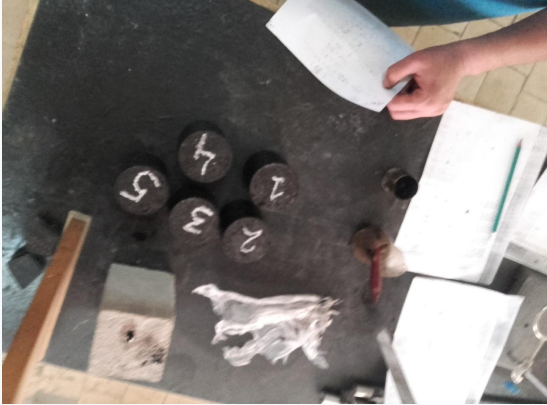
Picture 2. The process of making asphalt concrete samples
