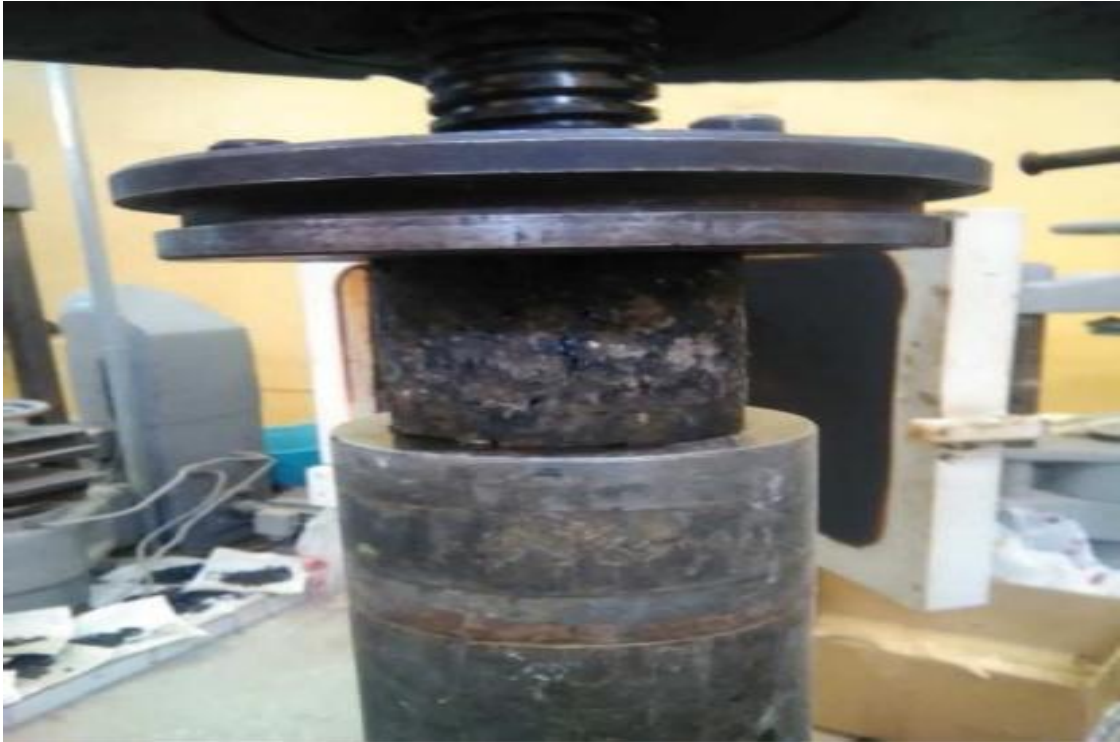
The dependence of samples on the strength and content of the samples. Table 2 Picture 1. Process of verification of prepared asphalt concrete in hydraulic press.
