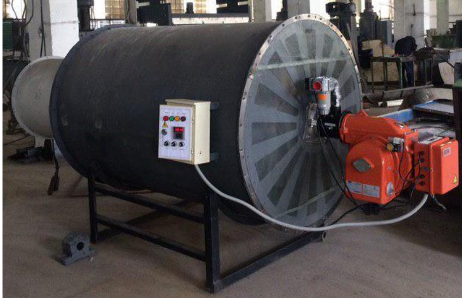
Fig. 2. General view of the developed and manufactured heat generator TGU
