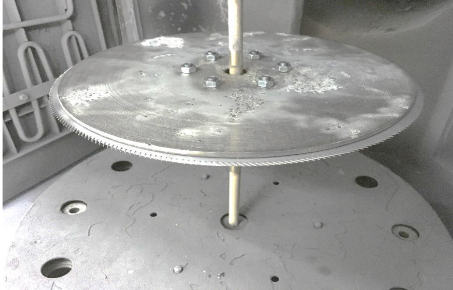
Fig.2. Disk saw with snap-in, placed in the vacuum chamber of the installation "STANKIN-APP-1".
