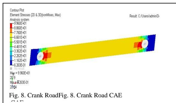
When all components pass in the CAE with Minimum Factor of safety 1 the project is then proceed to the fabrication stage. For providing movement to the mechanism I used the DC Wiper Motor of car because of its low rpm and high
