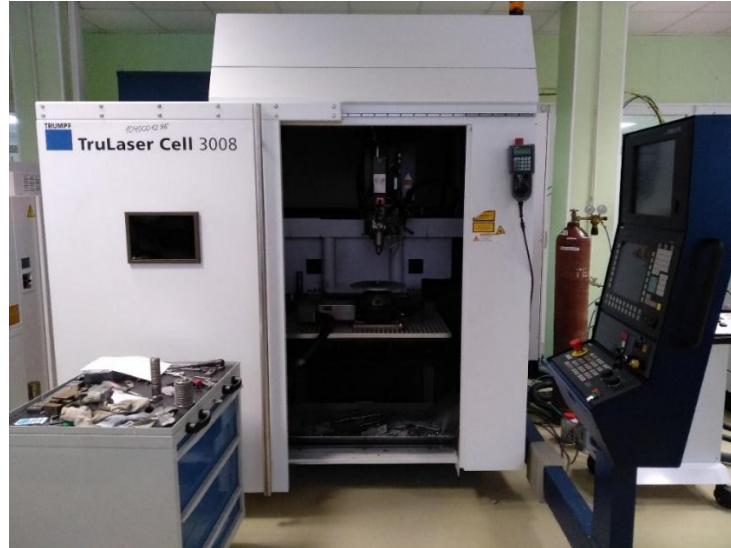
Fig.2. 5-coordinate laser processing center TRUMPF TruLaserCell 3008 LMD.
