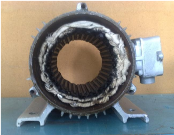
Figure 1. The stator of a periodic pulse voltage machine generator
