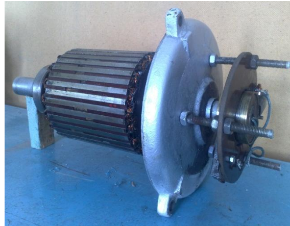
Figure 2. The rotor of a periodic pulse voltage machine generator with a brush mechanism
