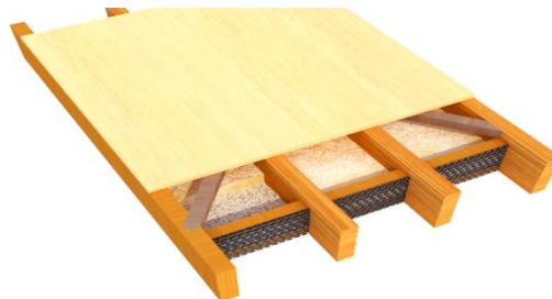
Figure 1. An overview of innovative lightweight and energy-efficient panel construction for roofing and interspace covering.
