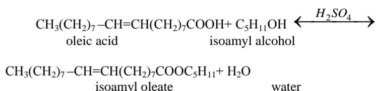
In this regard, the synthesis of ether was carried out at a temperature of 140 ° C, the duration was 0.5 hours, the catalyst was 0.5% (by weight of the mixture) and in various initial ratios of acid and alcohol.
