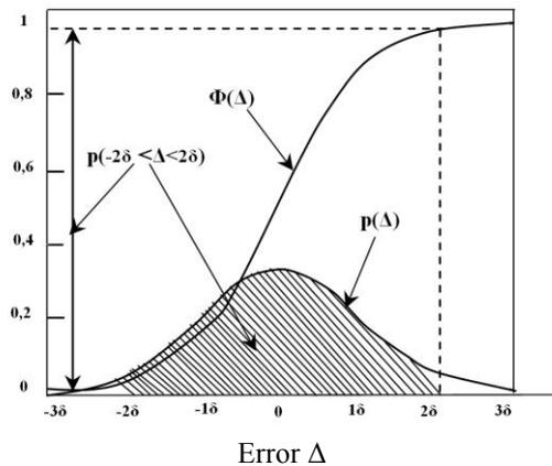
Here,  $\Delta$  is the measurement error;  $P(\Delta)$  is the density of the distribution of errors  $\Delta$ ;  $\Phi(\Delta)$  is the error distribution function:
