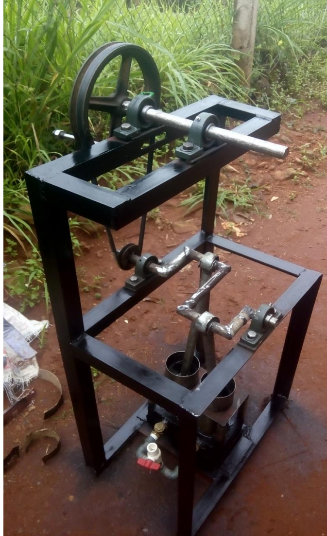
Figure 2: The fully constructed hand operated water pump
