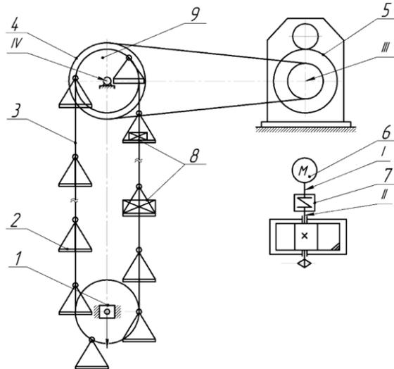
1-tension device; 2-cradle; 3-load chain; 4-chain transmission; 5-cylindrical gearbox; 6-engine; 7-elastic sleeve-sleeve coupling; 8-load; 9-chain load chain I, II, III, IV - shafts, respectively, of the engine, high-speed and low-speed gearbox, working machine
