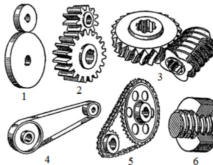
1-friction cylindrical; 2-gear cylindrical; 3-worm; 4-belt; 5-chain; 6-threaded chassis
