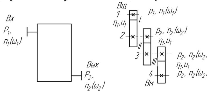
Fig. 1. Transmission scheme with series-connected links
