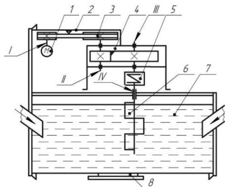
1-engine; 2-fence; 3 V-belt drive; 4-cylindrical gearbox; 5-elastic coupling with a mountain shell; 6-stirrer; 7-mixture; 8-valve I, II, III, IV - shafts, respectively, of the engine, high-speed and low-speed gearbox, working machine
