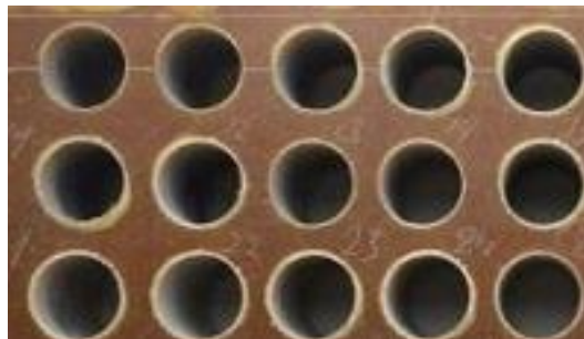
Fig. 4 Sample for examining bundles and chip stacking.
