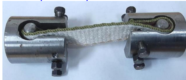
Picture-2. Device for fastening the tape during the tear test.
