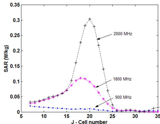
Fig.8. SAR distribution of eye with frequency
