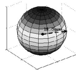
Fig.7. Eye model for SAR evaluation
