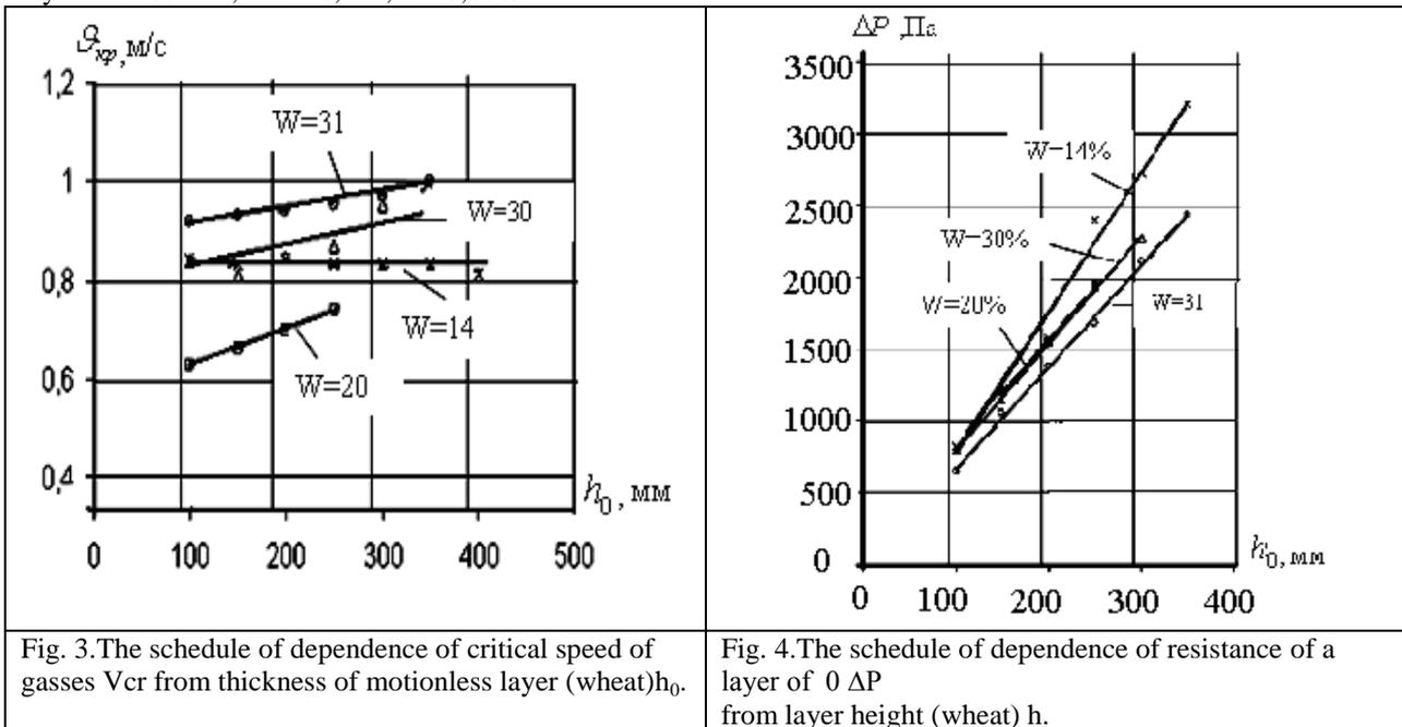
Thus, the received results of research of model disperse materials give the chance to estimate energy expenses at IBL (the intensified boiling layer) at the beginning of thermal processes (drying, gasification, burning, etc.) falling on a certain productivity of production and to choose the fan.
