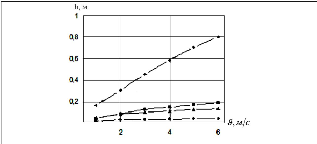
Fig 7. Dependence of change of height of a layer of hon the speed of gasses of mix  $g$ :  $K= 0,35$ ;  $K= 1$ ;  $K= 2$ ;  $K= 3$
