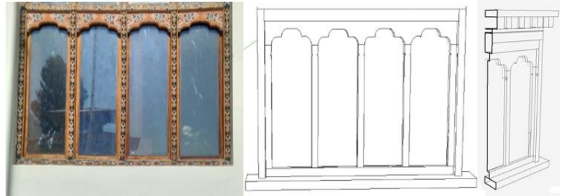
Figure 15: Front elevation of the selected window
