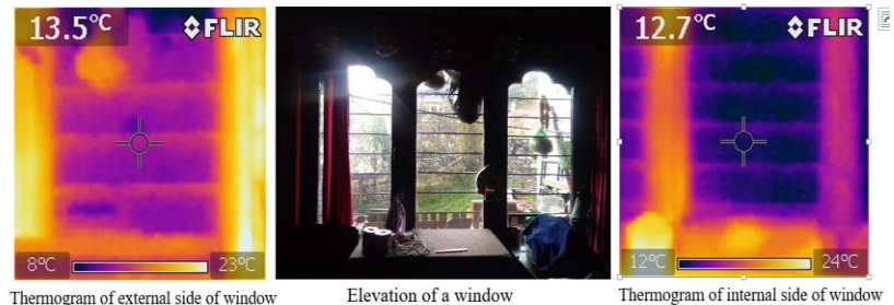
Figure 20: Thermogram of window surface
