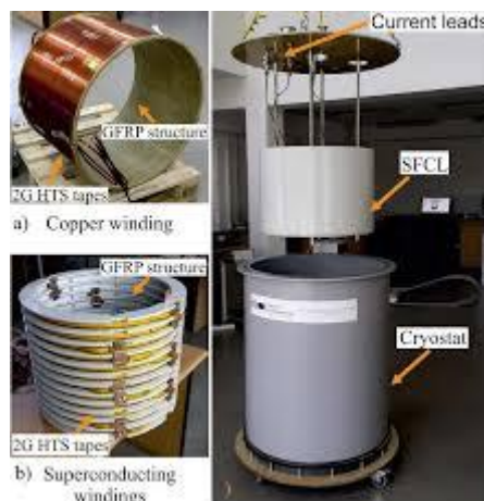
Fig. 2. Coreless inductive superconducting fault current limiter with winding made of Super Power SF12050 second Generation superconducting tape
