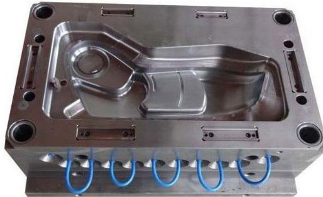
Fig. 2. Development of mold parts for control programs in NX CAM.
