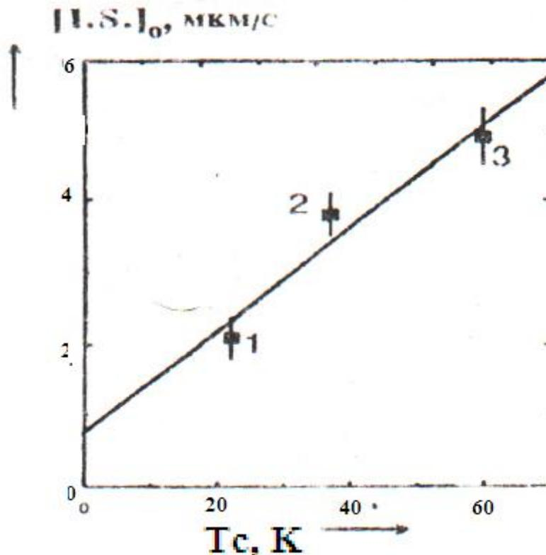
Fig. 3, Temperature dependences of the center of gravity  $S$  of the Mossbauer spectrum of  $^{67}Zn$ , measured relative to its value at 37 K, for  $La_{1.85}Sr_{0.15}^{67}CuO^4$  (1);  $La_{1.85}Sr_{0.15}CuO_4$ :  $^{67}Ga$  (2) and  $^{67}Cu_3O$  (3). The theoretical temperature dependence of  $S$  is given for the case of the second-order Doppler shift at  $\theta = 400$  K.
