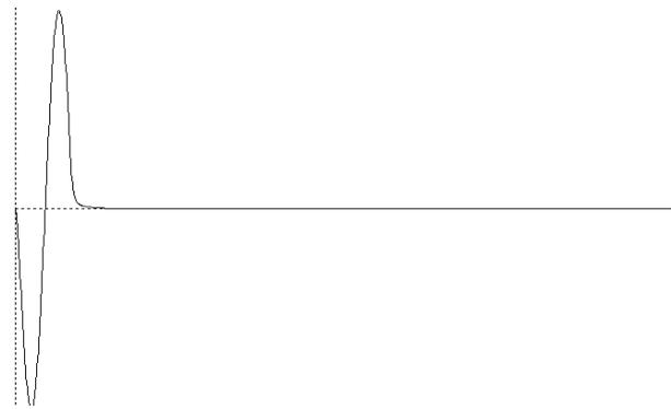
Figure 3. Change in shear forces at  $x=0.5$  m over time, the maximum value is 61000 N
