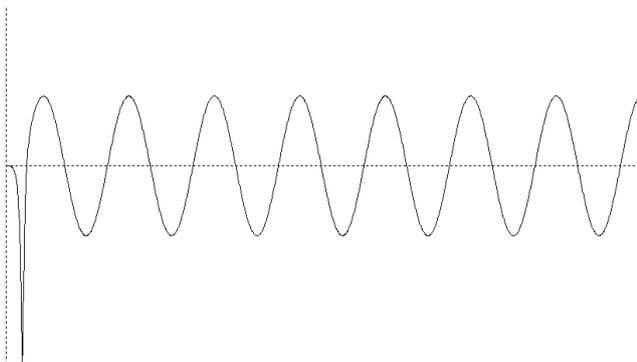
Figure 5. Change in moments of force at the point  $x=19.5$  m over time, the maximum value is 3220 Nm, the stationary maximum value is 1100 Nm
