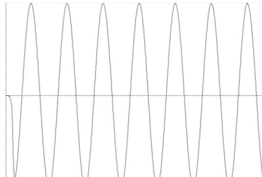
Figure 6. Change in shear forces at  $x=19.5$  m over time, the maximum value is 50300 N, the stationary maximum value is 56200 N
