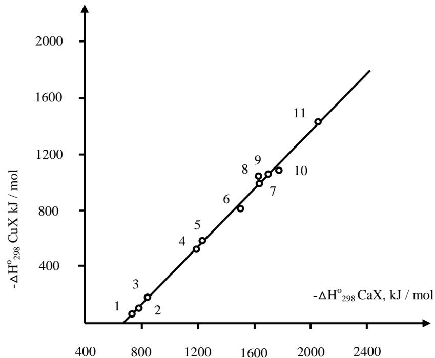
**Fig.1.** Comparison of the standard heats of formation of crystalline copper compounds and calcium (M = Cu or Ca): 1-  $M(\text{ClO}_3)_2$ , 2-  $M(\text{ClO}_4)_2$ , 3-  $M\text{Cl}_2$ , 4-  $M\text{SeO}_4$ , 5-  $M\text{SO}_3$ , 6-  $M\text{SO}_4$ , 7-  $M\text{MoO}_4$ , 8-  $M\text{Fe}_2\text{O}_4$ , 9-  $M\text{SeO}_3 \cdot 2\text{H}_2\text{O}$ , 10-  $M\text{WO}_4$ , 11-  $M(\text{HCO}_3)_2$ .
