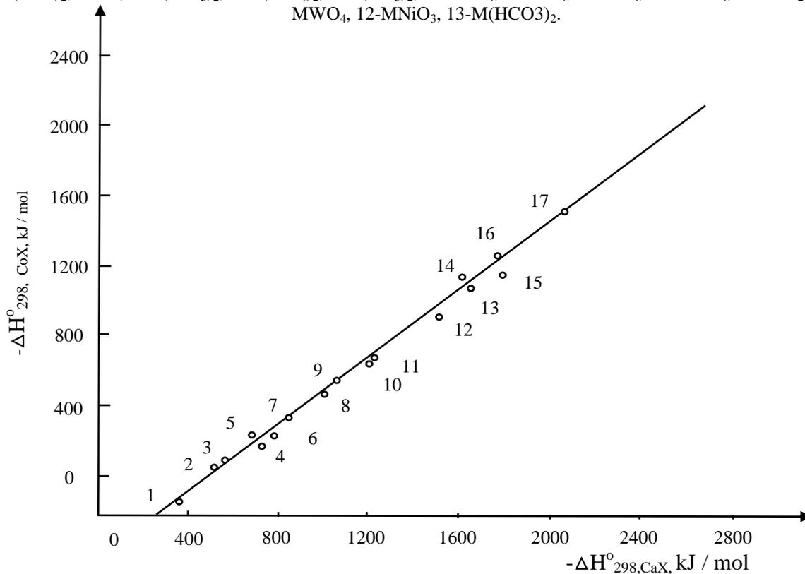
**Fig. 3.** Comparison of standard heats of formation crystalline cobalt and calcium compounds (M - Co or Ca): 1-  $M(\text{CNS})_2$ , 2-MS, 3-MI<sub>2</sub>, 4- $M(\text{ClO}_3)_2$ , 5-MO, 6- $M(\text{ClO}_4)_2$ , 7-MCl<sub>2</sub>, 8- $M(\text{NO}_3)_2$ , 9- $M(\text{OH})_2$ , 10-MSeO<sub>4</sub>, 11-MSO<sub>3</sub>, 12-MSO<sub>4</sub>, 13-MMoO<sub>4</sub>, 15-MWO<sub>4</sub>, 16-MTiO<sub>3</sub>, 17- $M(\text{HCO}_3)_2$ .
