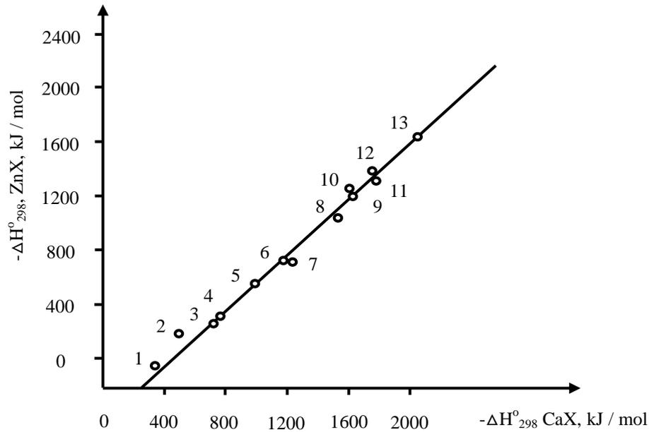
**Fig. 2.** Comparison of the standard heats of formation of crystalline zinc and calcium compounds (M=Zn or Ca): 1-  $M(\text{CNS})_2$ , 2-MS, 3- $M(\text{ClO}_3)_2$ , 4- $M(\text{ClO}_4)_2$ , 5- $M(\text{NO}_3)_2$ , 6-MSeO<sub>4</sub>, 7-MSO<sub>4</sub>, 8-MSO<sub>4</sub>, 9-MMoO<sub>4</sub>, 10-MFe<sub>2</sub>O<sub>4</sub>, 11-MWO<sub>4</sub>, 12-MNiO<sub>3</sub>, 13- $M(\text{HCO}_3)_2$ .
