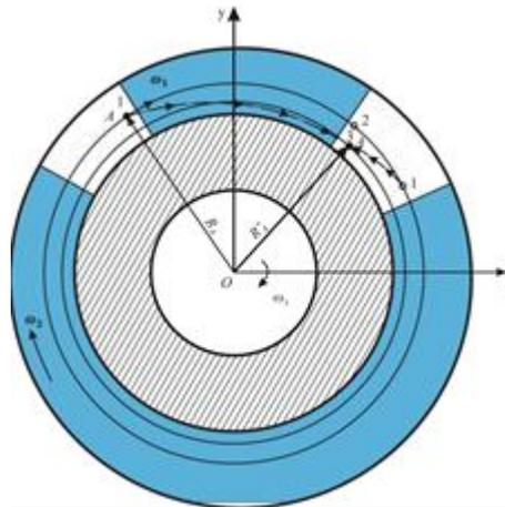
It is extremely important that heavy particles in the loaded stream will tend to the axis of rotation. A diagram of such a dynamics of heavy particles is shown in Figure 1.
