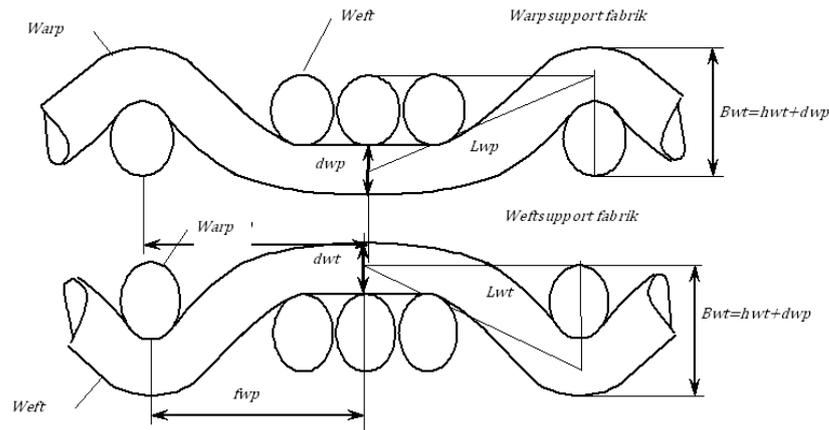
Fig.1. The cuts tissue along the warp and weft
