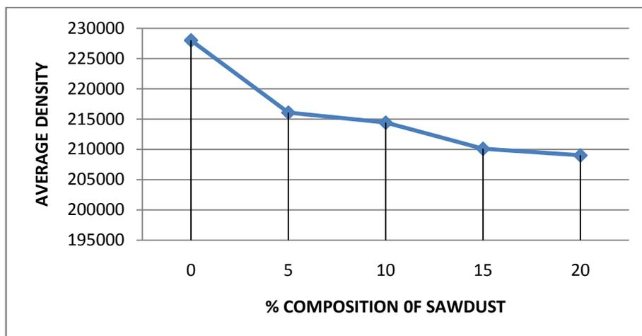
Fig. 2: Relationship between density of the specimens and sawdust content
