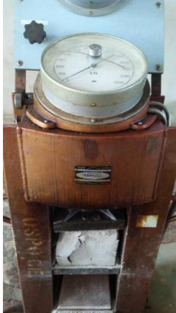
Fig. 3: Universal compression Testing Machine
