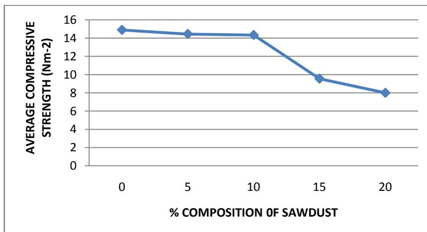
Fig. 4: Relationship between compressive strength of the specimens and sawdust content
