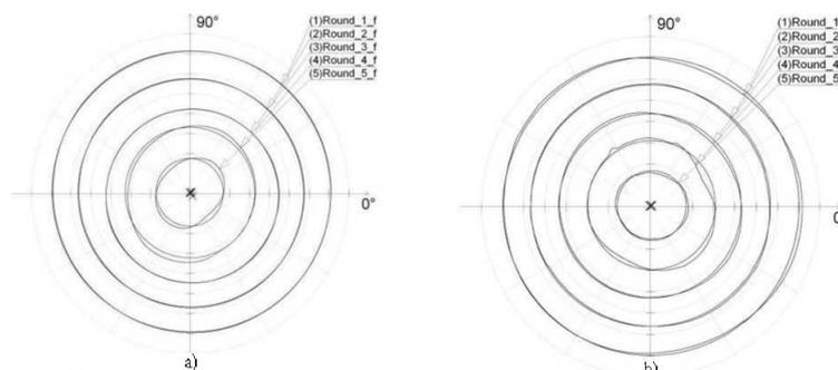
Figure 5. Roundness deviation of the shaft-puller: a) turning of the shaft with tensile force; b) machining without tension, at normal turning
