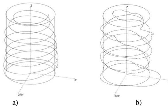
Figure 4. Cylindricity deviation of the shaft-puller: a) turning in the elastically deformed state; b) at normal turning
