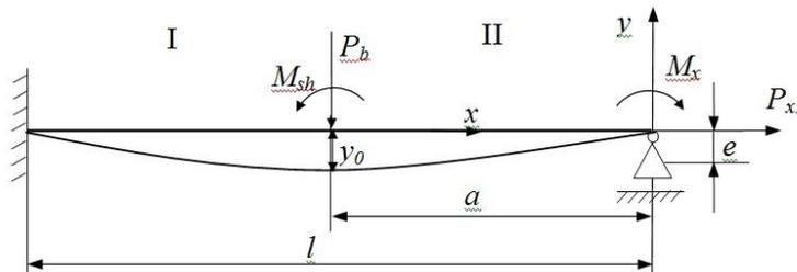
Figure 2. Calculation scheme of stresses and elastic line of the shaft by stretching:  $e = 0.001$  – eccentricity of stretching force putting;  $M_{sh}$  – cutting forces moment;  $M_x = P_{xl} \cdot e = 34.822 \cdot 0.001 = 0.034822 \text{ Nm}$  – tensile stress moment
