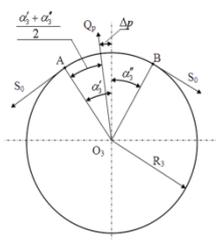
Fig. 4. The calculation scheme of the interaction belt with the compound tension roller
