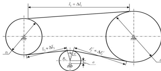
Fig. 2. Belt drive scheme with eccentric tensioning roller
