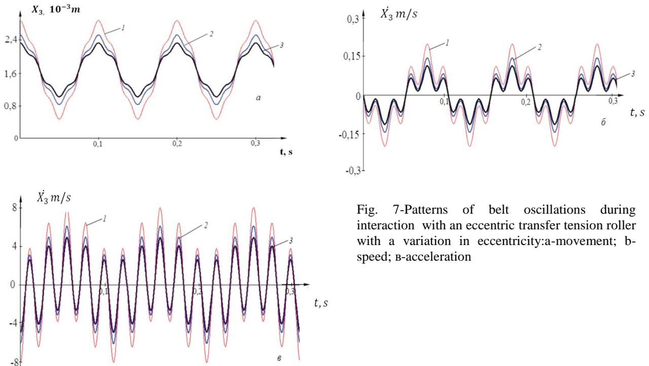
Fig. 7-Patterns of belt oscillations during interaction with an eccentric transfer tension roller with a variation in eccentricity: a-movement; b-speed; c-acceleration
