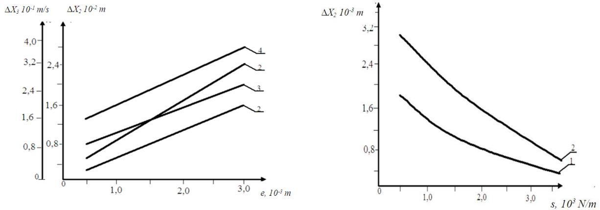
Fig. 8- The pattern of changes of  $\Delta X_2$  with the variation of displacement and the stiffness coefficient of the elastic plug of the tension pulley of the driven belt
