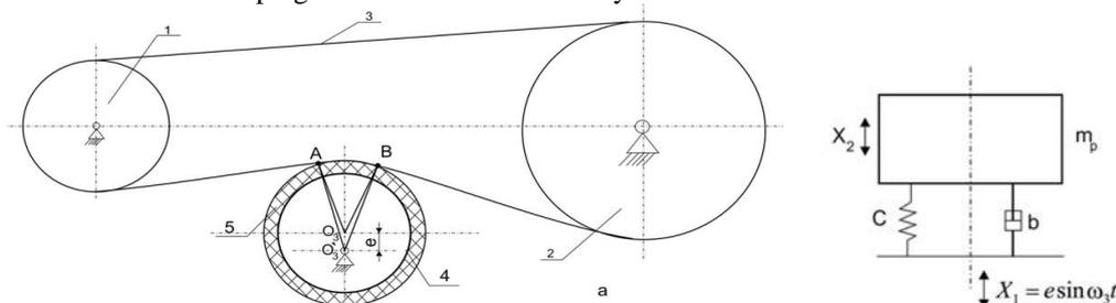
Fig. 6: a-kinematic scheme of belt drive with compound eccentric tensioning roller; b - the calculate scheme of oscillations the part of a driven path of a transmission belt
