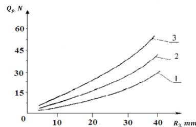
Fig.5. The pattern of change in the interaction force of the tension compound roller with the belt at the variation of the radius in the tension roller
