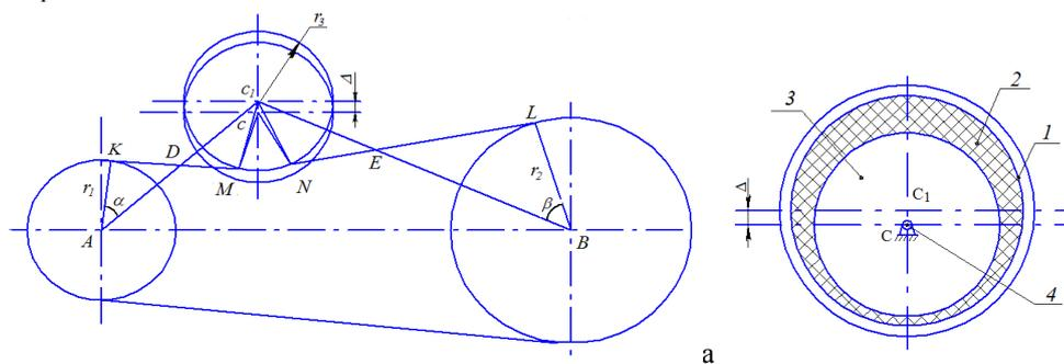
Fig. 9. a- Scheme of the belt drive with a compound tension roller, b - tension roller, with a shifted position of the outer plug due to deformation of the elastic plugs 2
