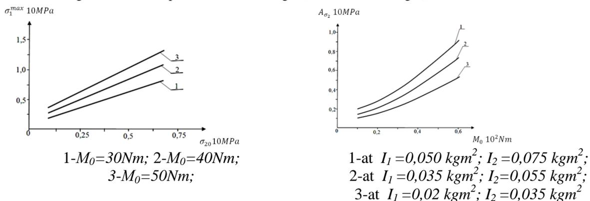
Fig. 3. The pattern of change in the maximum value of the tension in the driven path of the belt transmission from the change tension with the preloading of the driven path (a) and the amplitude of the oscillations tension in the driven path of the transmission from the variation  $M_0$
