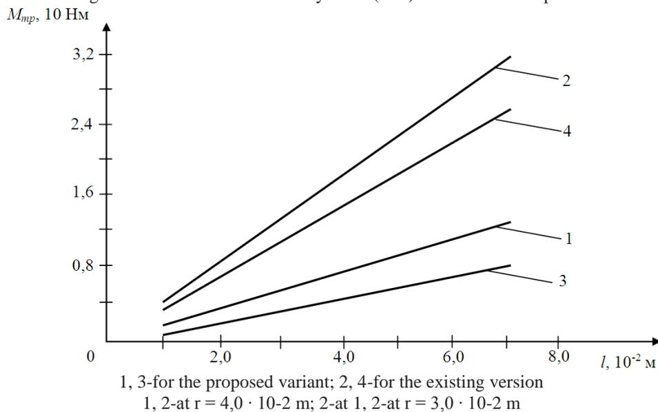
Fig. 4. Comparative dependence of the change in the torque on the frictional forces on the change in the length of rotational kinematic pairs
