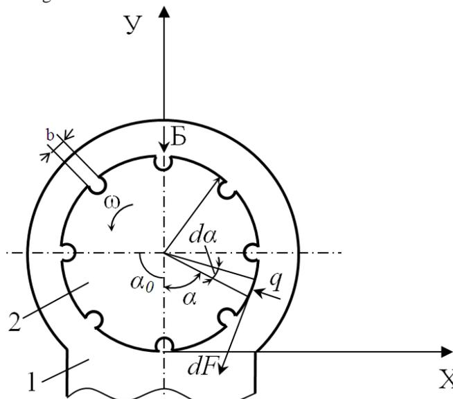
1-axis (cylinder), 2-pin (housing)
