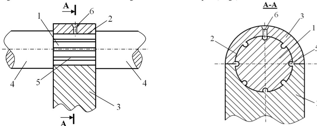
Fig. 1. Rotary kinematic pair of the fifth class with longitudinal grooves of the axis
