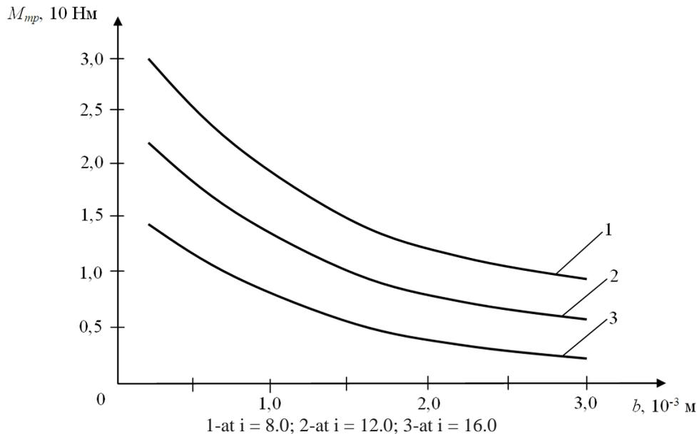
Fig. 3. Graphical dependences of the change in the torque of the frictional force on the width of the longitudinal grooves on the surface of the cylinder (axis) of the kinematic pair
