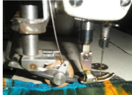
b-the process of applying the polymer composition to the lines
