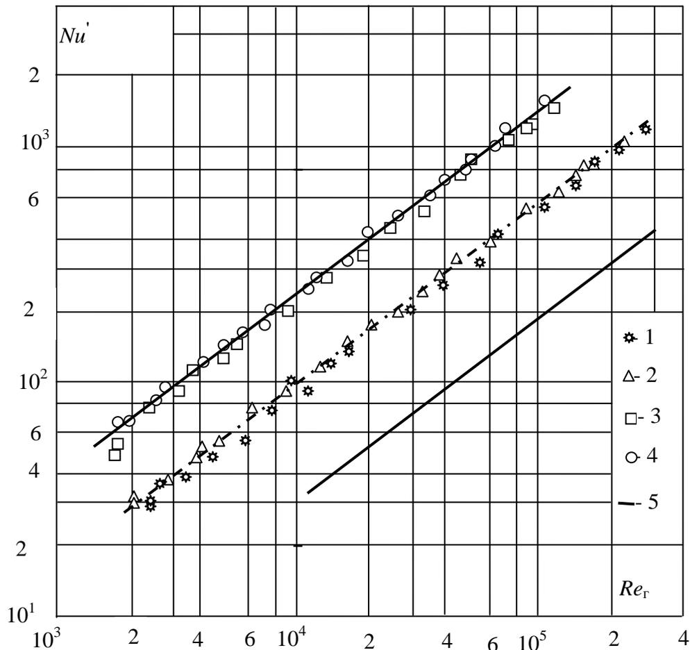
**Fig. 2.** Dependence of the Nusselt diffusion criterion on the Reynolds number
