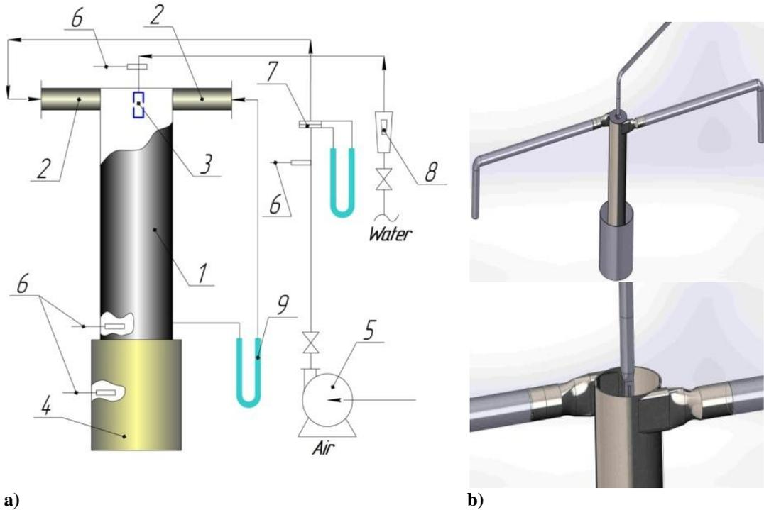
**Fig.1.a** - The scheme of the experimental setup; **b-** 3D view of the experimental setup;
