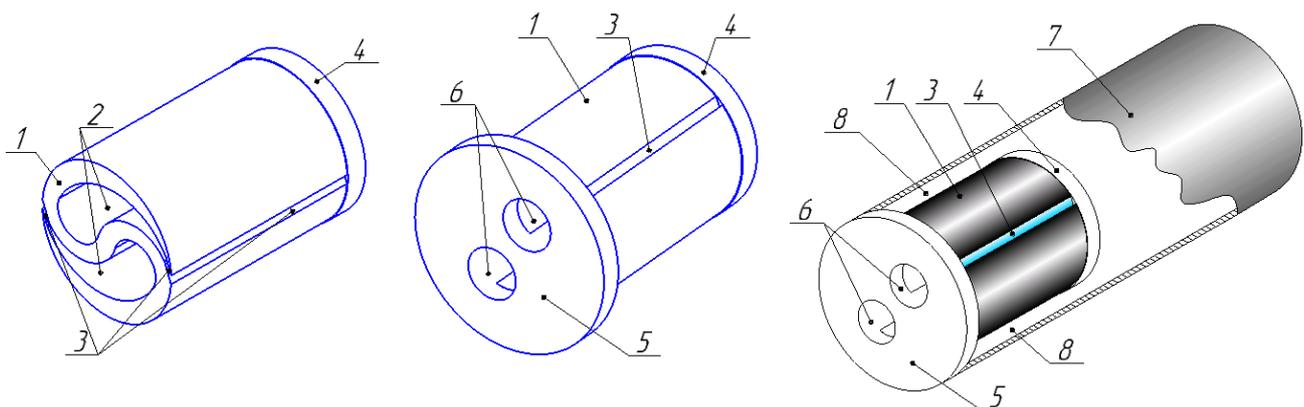
**Fig. 2. The swirler assembly in the apparatus (in the tube)**
