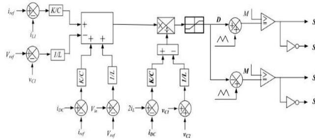
Fig.2.Sliding Mode control Modelling
