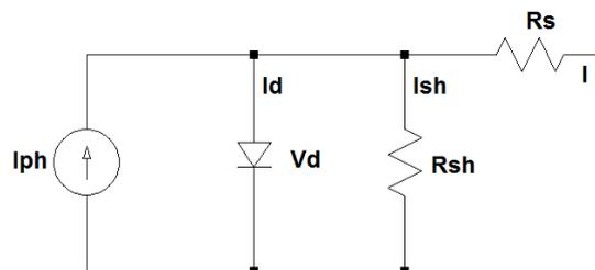
Fig.3. Basic diagram of Solar PV Cell
