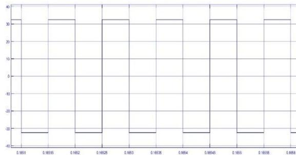
Fig.5. Output voltage of Quasi Z-Source Inverter using SMC
