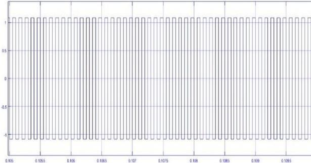
Fig. 6. Output current of Quasi Z-Source Inverter using SMC
