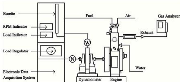
**Fig 4.1: The Schematic Diagram of Experimental Setup**
