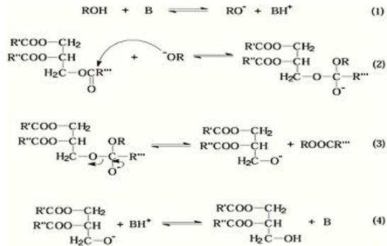
Fig.2.1 Mechanism of base catalysed Transesterification
