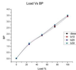
Figure 5.1 shows the variation of brake power with respect to load for diesel fuel and Karanja biodiesel and additives .it can be observed from the figure that shows that there is no significant change in brake power .All blends i.e B10,B20, B30 including diesel gave more or less same readings. In specific 6% loss in Brake power is observed, this is because of low energy content of karanja blends.
