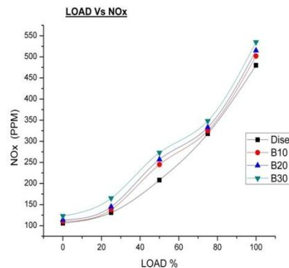
Figure 5.9 shows the variation of NOx with respect to load for diesel fuel and Karanja biodiesel and additives. Due to the excess oxygen present in the biodiesel complete combustion took place and temperature inside the combustion chamber increased thereby increasing the NOx emission. From the graph it is clear that B30 showed maximum NOx emissions. It cannot be completely stopped but it can be minimized like EGR techniques.
