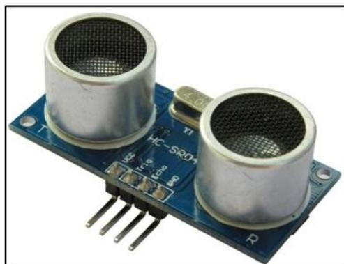
**Figure 2 Ultrasonic Sensor HRSO4**
