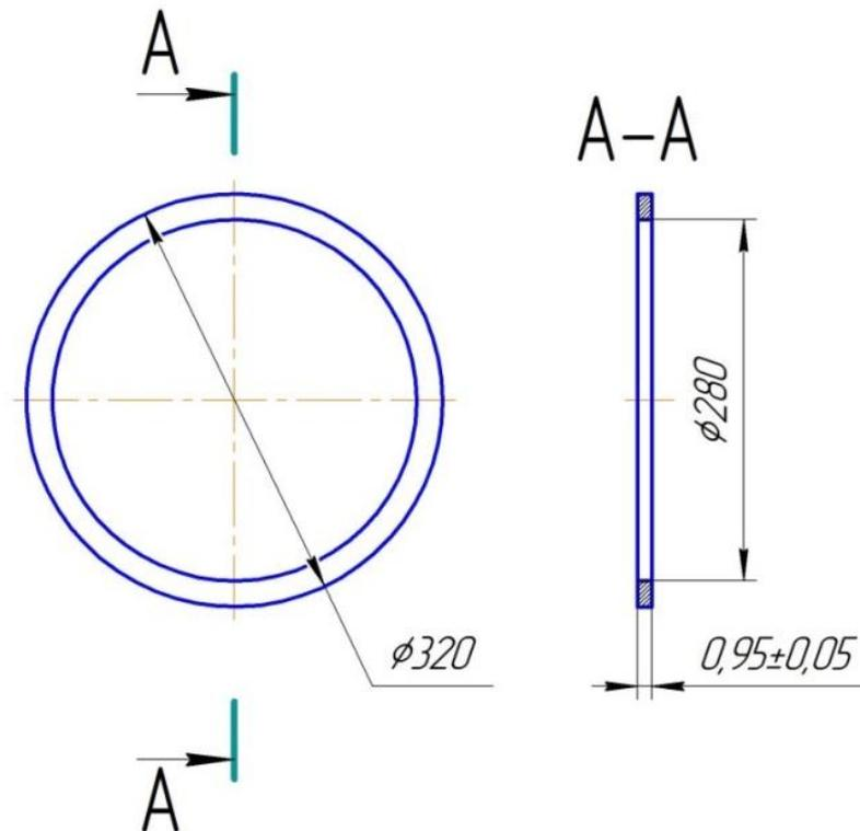
Fig. 2. Parameters of specimens-rings subjected to heat treatment.
