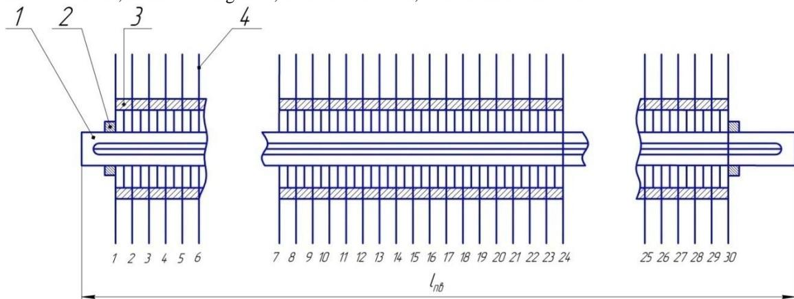
Fig. 5. Scheme of assembling a new design equipped with circular saws of the experimental unit of the saw cylinder.
