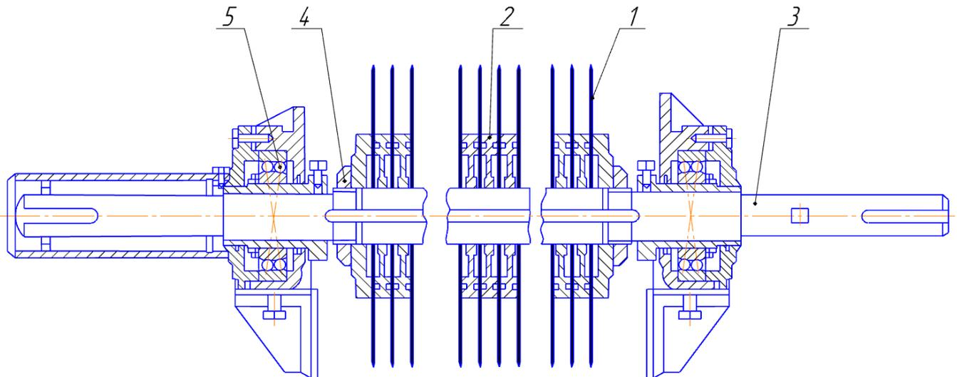
Fig.1. Design of the assembly of the saw cylinder of the fiber separating machine.
