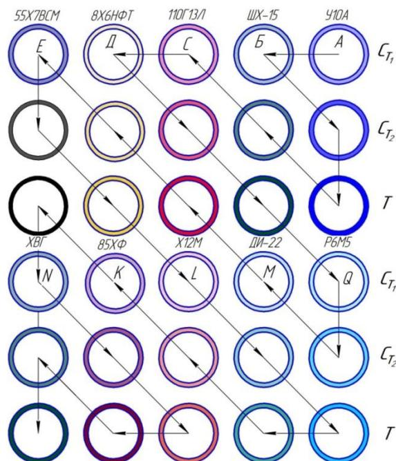
Fig.4. The scheme of randomization of ring samples by the method of "diagonals"
