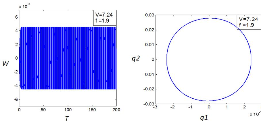
Fig.1 The time-domain curve and phase diagram of the flexible beam when  $V < V_{div-dy}$  ( $V=7.24, f=1.9$ )
