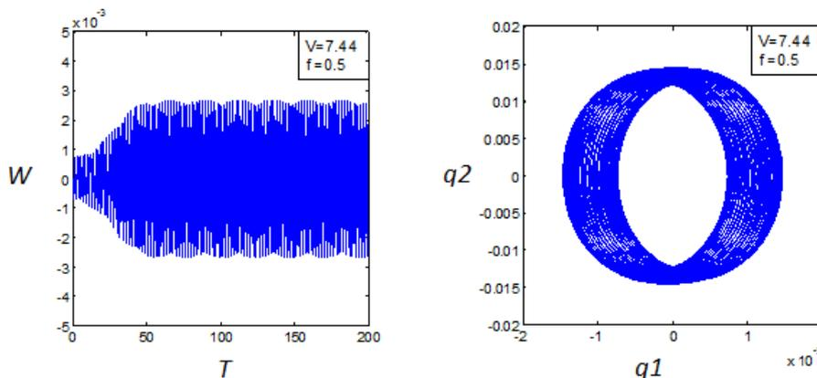
Fig.2 The time-domain curve and phase diagram of the flexible beam when  $V < V_{div-dy}$  ( $V=7.44, f=0.5$ )
