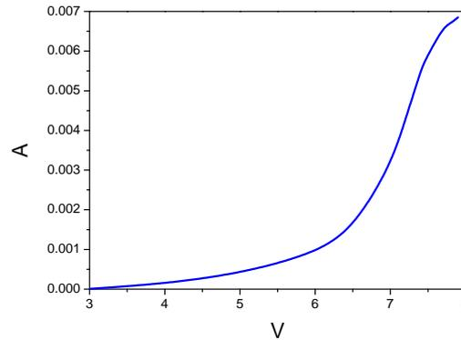
Fig.3 The effect of flow velocity on vibration response amplitude
