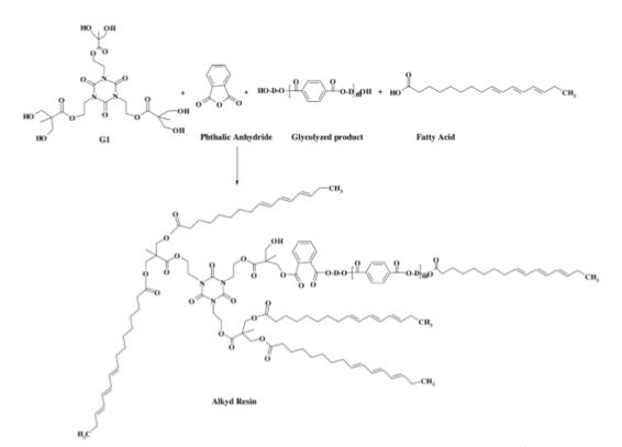
Fig 4: Alkyd resins from PET waste and Bio-derived fatty acids of oils <sup>(6)</sup>
