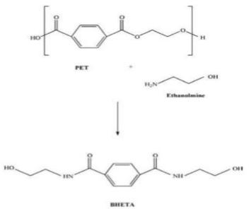
Fig 3: Aminolysis of PET waste <sup>(3)</sup>
