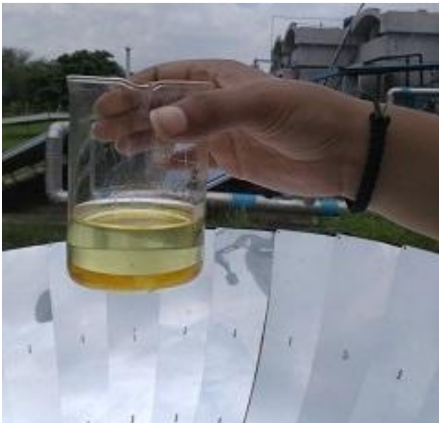
2(e) Prepared crude biodiesel after transesterification
